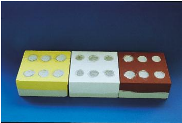
Cohesive failure after adhesion tests
